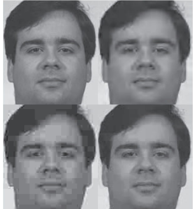
Fig. 5. Qualitative evaluation of ITAD codec. Clockwise from top-left: original, JPEG2000 (0.31 bpp, 31.46 dB), ITAD codec (0.31 bpp, 33.90 dB) and JPEG (0.33 bpp, 29.15 dB).
