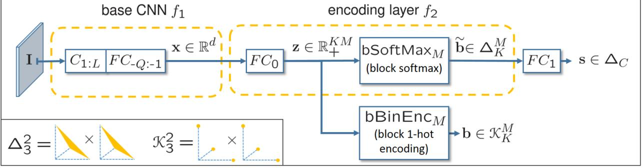
Figure 1: **Proposed architecture and notations.** A feature is extracted from image  $\mathbf{I}$  by a base CNN  $f_1$  and binarized using a block-structured encoding layer  $f_2$  consisting of a fully-connected layer followed by a *block softmax* during training, or a *block 1-hot encoder* during testing.
