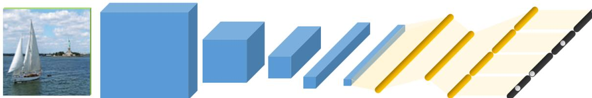
We introduce SUBIC, a *supervised structured binary code* (concatenation of one-hot blocks). It is produced by a novel supervised deep convolutional network and is well adapted to efficient visual search, including category retrieval for which it outperforms the state-of-the-art supervised deep binary hashing techniques.
